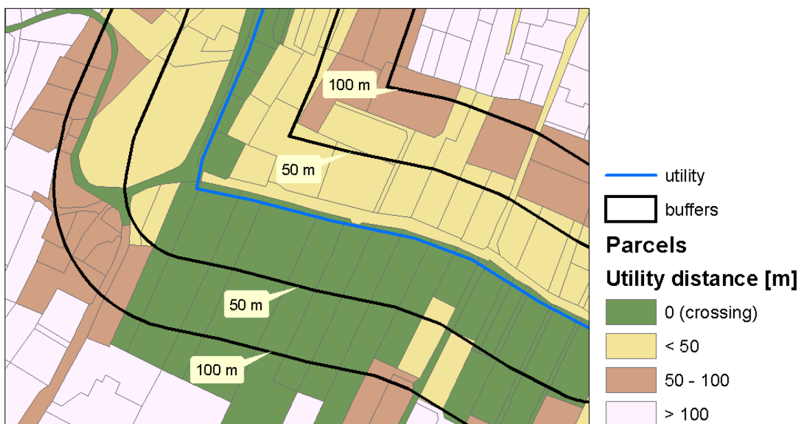
Figure 7. Buffer zones around utility.
