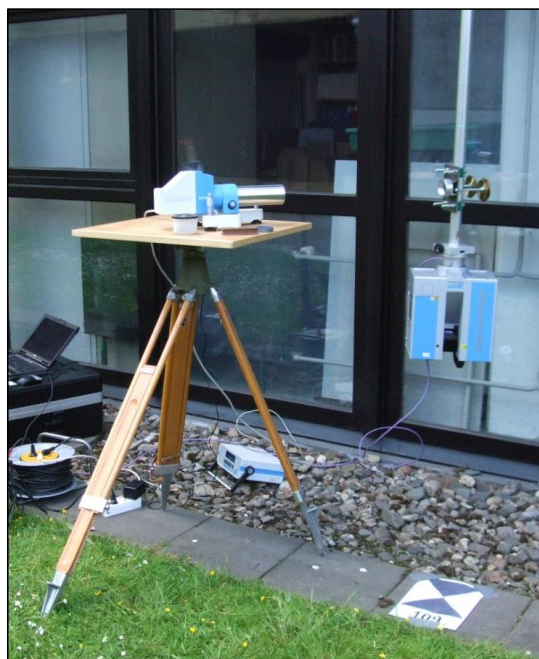
Fig. 6: Measurement of the rotation of the scanner with auto collimation
