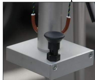
Fig. 5c: Adapter plate for the Scanner
