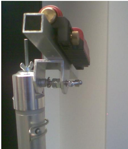
Fig. 4a: Laser pointer on the top of the tube elements
