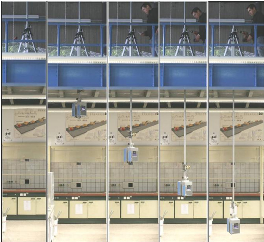
Fig. 7: Sequence of a measurement – the sewer is simulated by a hole in the balcony
