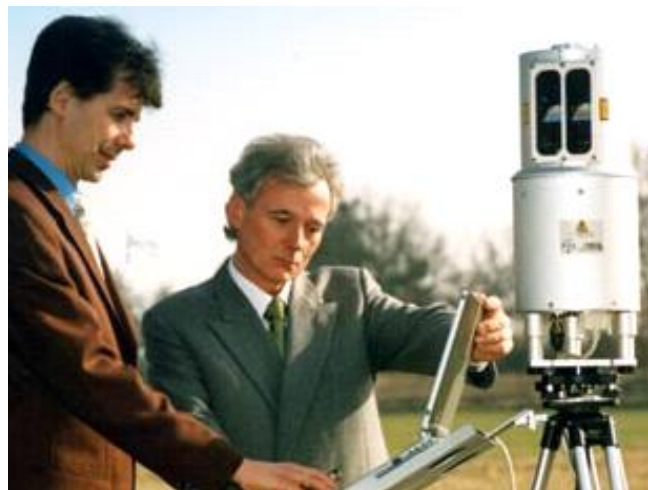
Fig. 1b: The first RIEGL Scanner LMS Z 210
