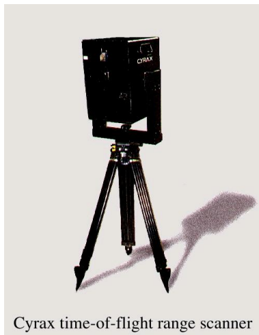
Fig. 1a: The first CYRAX-Scanner
