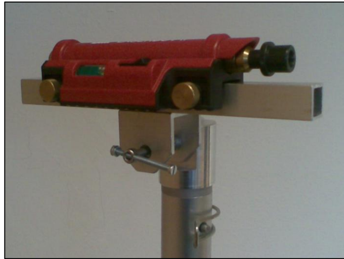
Fig. 4b: Laser pointer with a mechanical fixation for the inclination angle
