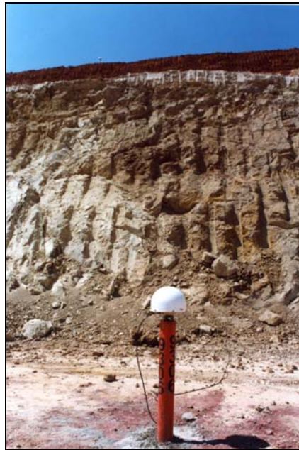
Fig. 1. Deformation station illustrating nearby high-wall which acts as a multipath reflector
