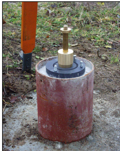
Figure 7: Reference point with insert tool in combined casing and tripod of Leica TC 1800
