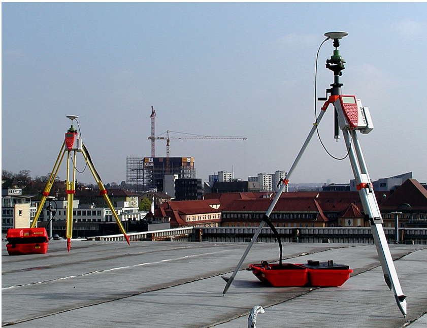
Figure 1: Measurement of baseline with PDGPS
