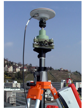
Figure 1: Measurement of baseline with PDGPS
