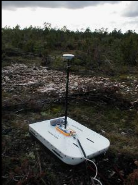
Mk1 with a Ground Penetrating Radar (GPR)
