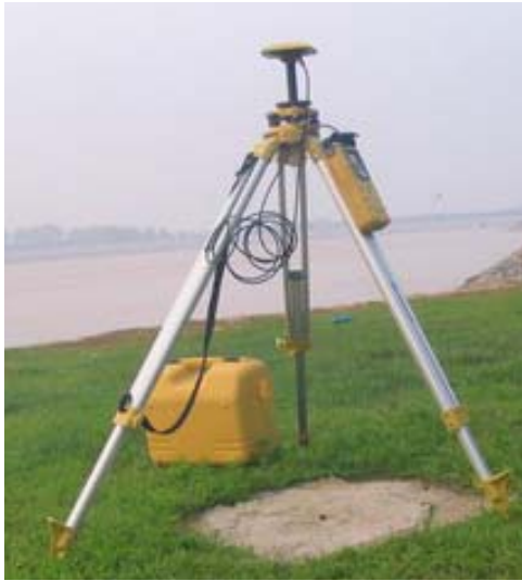
Figure 4: Conventional static GPS measurement
