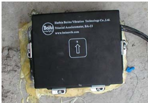
Figure 8: Triaxial accelerometer at the top of the tower Figure 9: Vertical accelerometer mounted on the bridge deck
