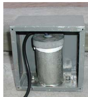
Figure 8: Triaxial accelerometer at the top of the tower Figure 9: Vertical accelerometer mounted on the bridge deck
