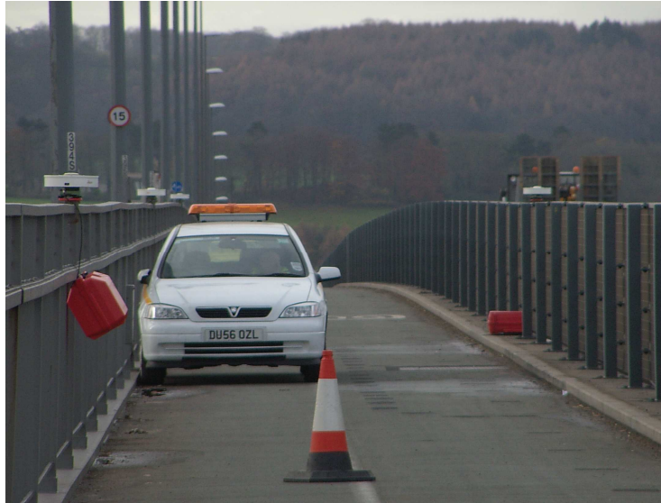
Figure 3 - Light-Weight Leica Choke Ring Antennas on Bridge Railings.
