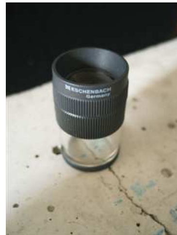
Figure 1 - Crack Template and Line Counter as classical devices for monitoring cracks
