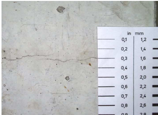
Figure 1 - Crack Template and Line Counter as classical devices for monitoring cracks
