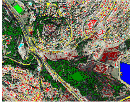
Figure 15: Change detection results – a comparison of satellite imagery and aerial photograph (Beit-Yaakov et al., 2003)
