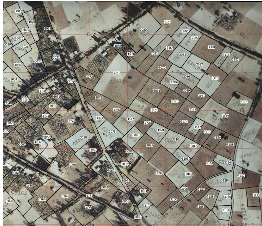
Vectorised field map showing the resulting cadastral map with parcel boundaries and cadastral numbers.
