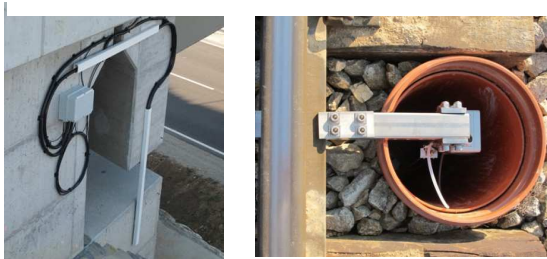
Figure 7 and Figure 8: Strain sensors and Rail-movement sensors installed at the bridge and rail
