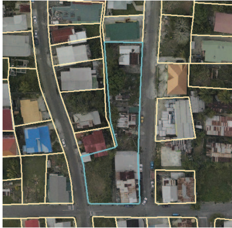
Figure 4. Legal boundaries conforming to physical boundaries of walls
