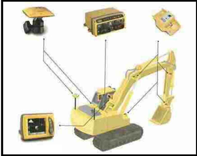
Machine control(MC) inclined sensor and GPS-independent surveying work
