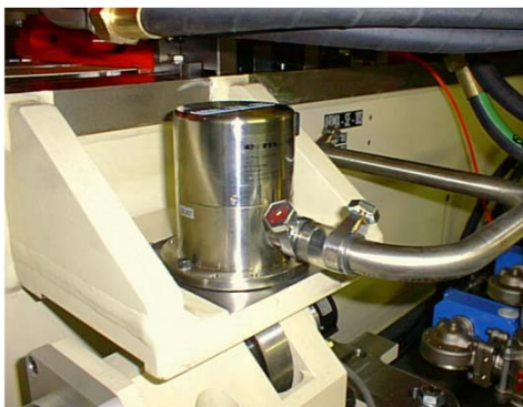
Levelsensor: Installation on girder
