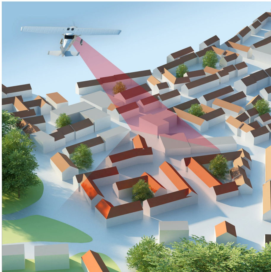
Figure 7: Air-borne detection of roof areas (Source: Prof. Dr. Martina Klärle, http://www.klaerle.de/ ).
