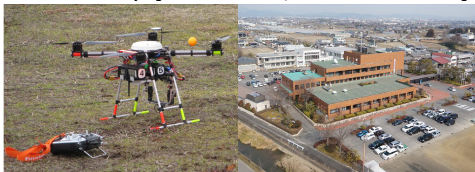
Fig. 5. UAV ( Multi- copter type) and oblique image ( Mizuho city – Sunami branch office )
