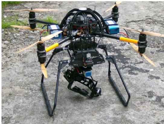
Figure 21 – Drone octocopter SKY II. The support of the camera is under the drone, between the landing gears.
