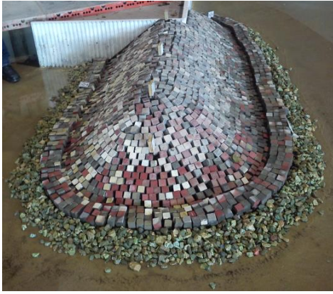
Figure 16 – Model of a breakwater.
