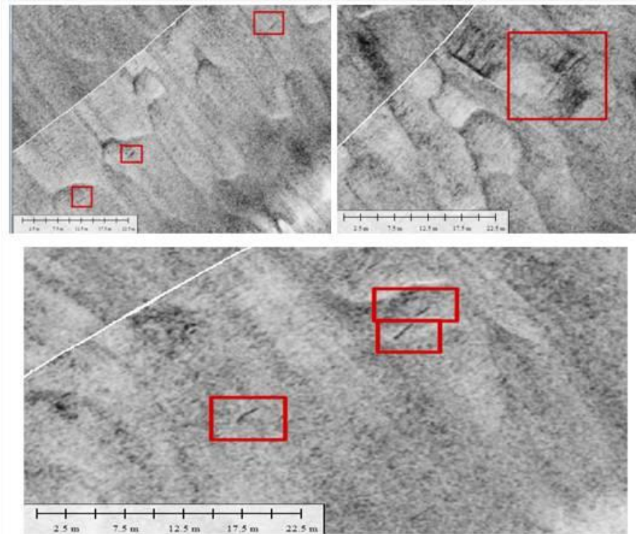
Figure 5. Red rectangles show location where cable section has been detected interpreting sidescan sonar data from most recent survey
