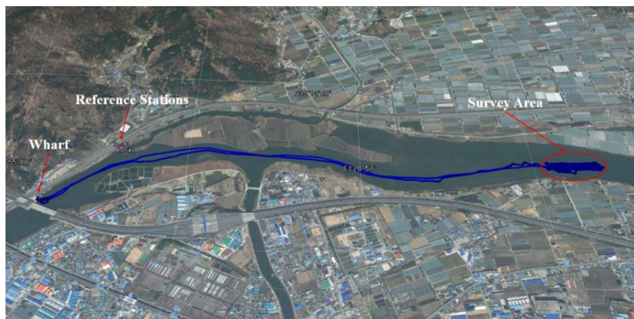
Figure 4. Trajectory of the survey vessel during the test with location of reference stations.
