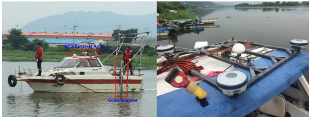
Figure 3. Surveying vessel and setup of GNSS receivers.
