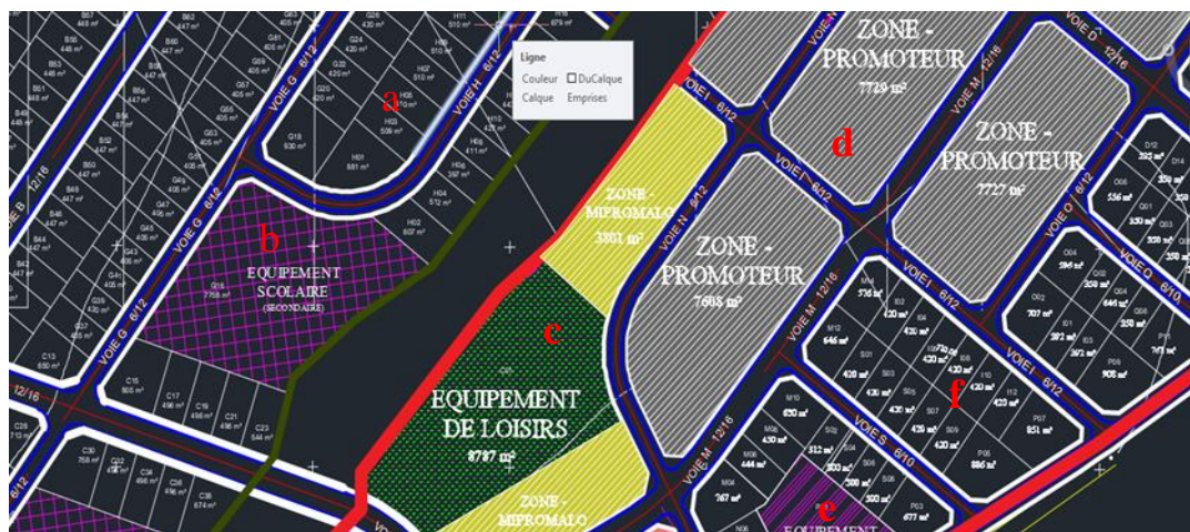
Figure 6: Example of needed organized parcels, Where a and f are spaces provide for housing facilities; b is a space allocating for school equipment; c space setting for leisure purpose; d space provide for urban developers; e allocating for health facilities. Source: MAETUR Nkondom Layout.
