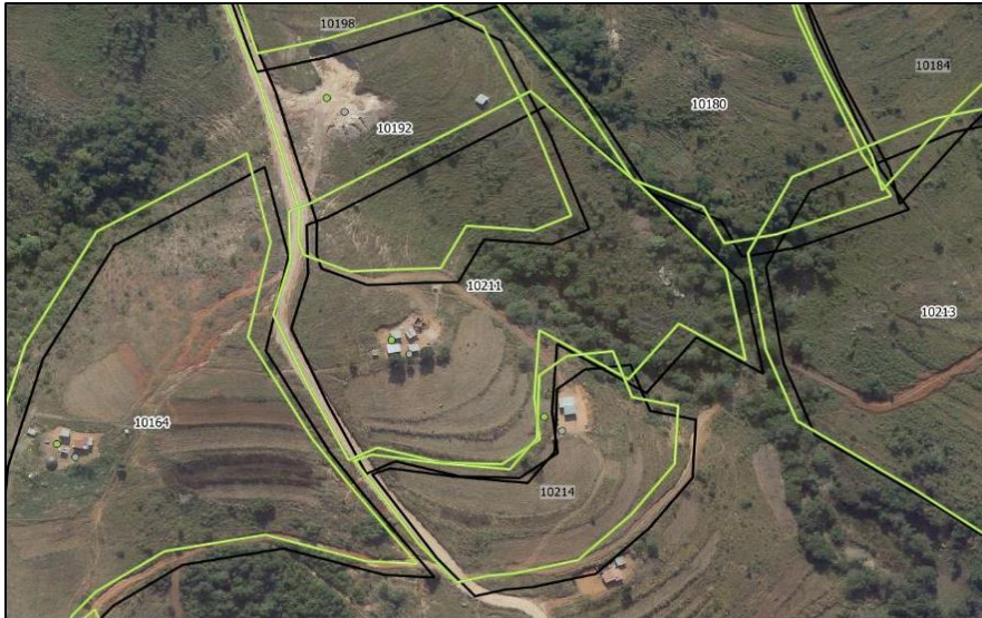
Figure 4: Unedited SLAM data (showing shifts between Lo (black) and WGS84 coordinate reference systems (green))
