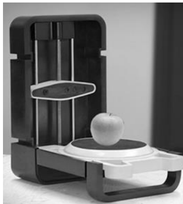
Figure 3 - The “Matter and Form” laser scanner used to determine the SA of a selected apple. The results from the scan were also used as an alternative method of computing the V.
