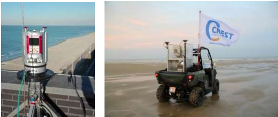
Figure 3: Long-range static and Mobile LIDAR for beach monitoring
