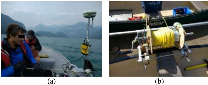
Figure 4. Options for a plate suspension mechanism: manual suspension via a pulley (a), and a custom-made gear reduction winch system with a spool
