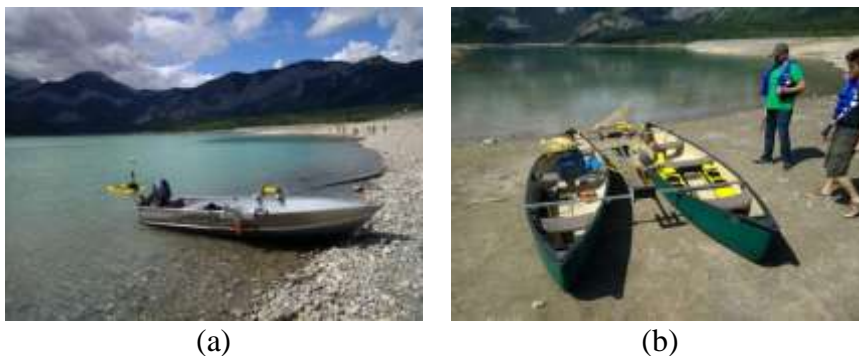
Figure 2. Options for a calibration platform: a fishing boat (a), and a two-canoe catamaran held together by an aluminum frame
