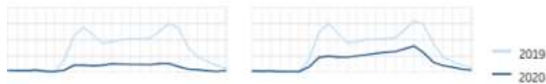
Figure 1 – Comparison between Travel Patterns as Average Congestion Level in April (left side) and May (right side) 2019 (light blue) and 2020 (dark blue), according with TomTom Data [10]
