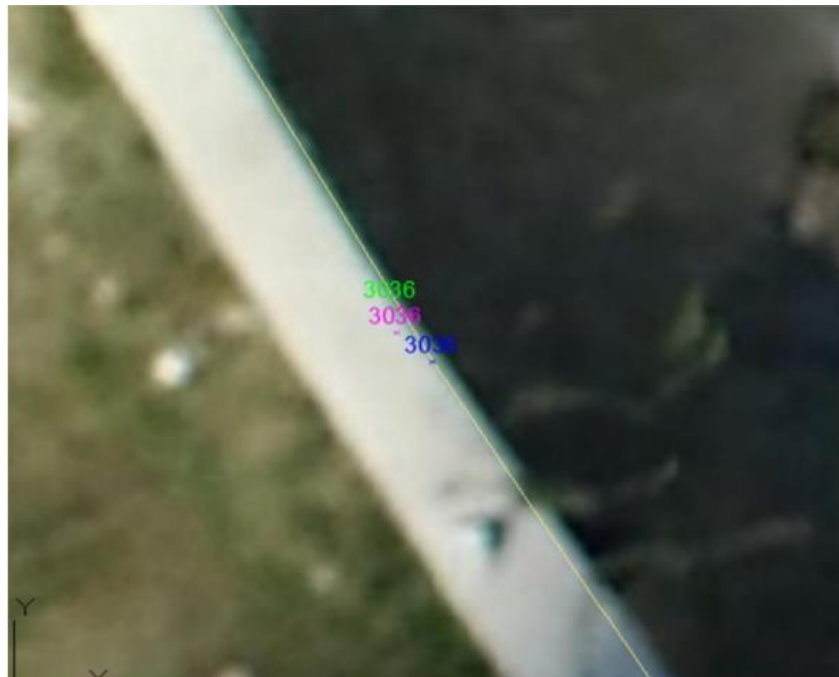
Fig 4. Delimitation differences between different survey techniques (blue: total station or GNSS, purple: mobile, green: static laser scanner survey) [1]
