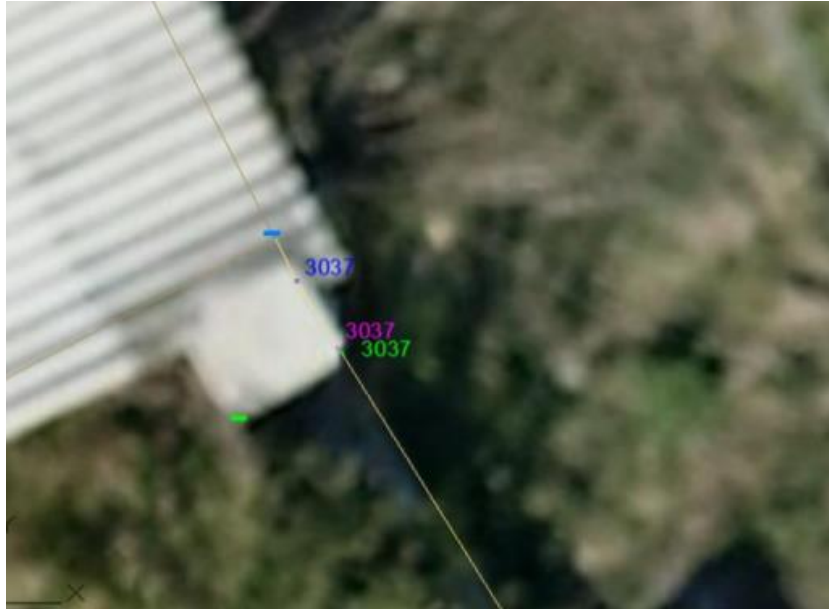
Fig 5. Delimitation differences between different survey techniques (blue: total station or GNSS, purple: mobile, green: static laser scanner survey) [1]
