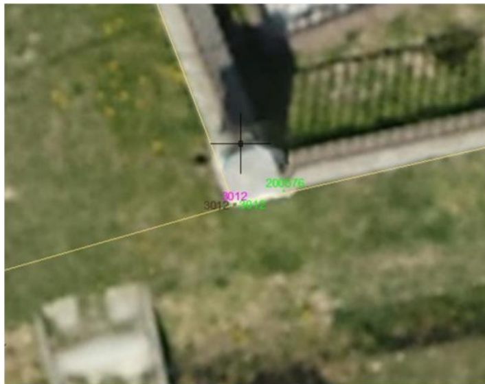
Fig 3. Points from different sources on an orthophoto extract (brown: traditional survey TS, GNSS, purple: mobile, green: static survey) [1]
