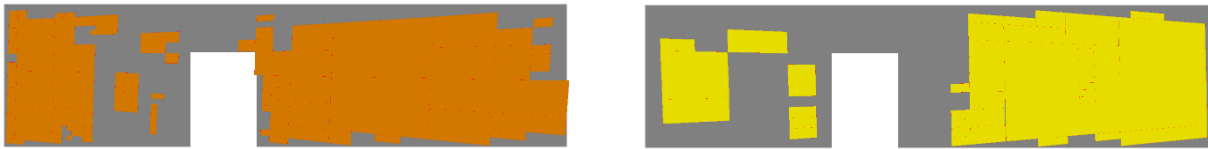
Figure 5: Visualization of the patches on a BIM face (grey) from 2 scanner stations
