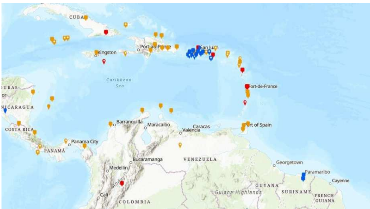
Figure 1: CORS in parts of Latin America and the Caribbean (United States National Geodetic Survey 2022)
