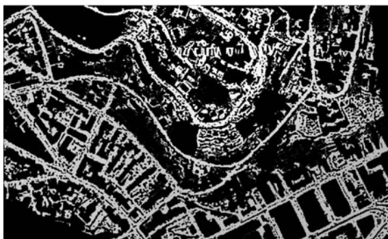
Figure 10. All data points used to calculate the final DTM
